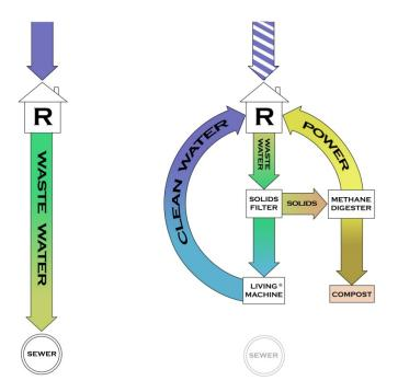
This diagram shows a comparison between the 'linear' water management of conventional buildings, and the cyclical system used in GROW Housing. nutrients within the wastewater are processed by the methane digester to produce both power and compost, while the Living Machine® filters the water to be used for all non-potable uses, including irrigation hydroponic farm.
