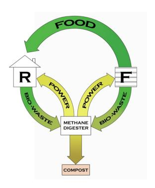
This diagram shows the relationship between the methane digester, vertical farm (F), and residential buildings (R). As the farm produces food for the residential units, large amounts of bio-waste are collected from the farm's production and fed into the methane digester to produce electricity, powering the artificial lighting of the farm. Additionally, the bio-wastes from the residents' usage of the food is directed to the methane digester, producing power for their homes.
